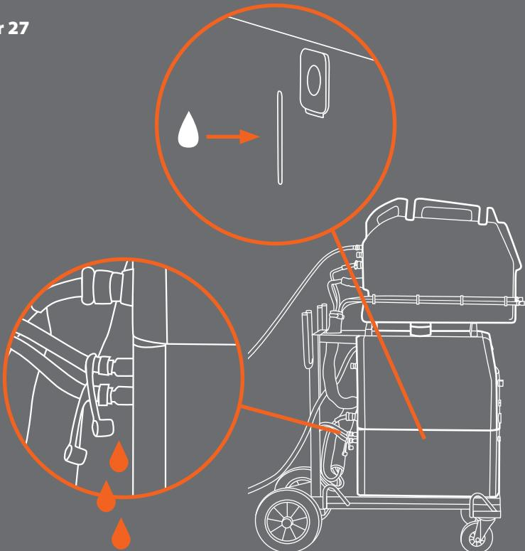
EN Check cooler function and cooling liquid level.
